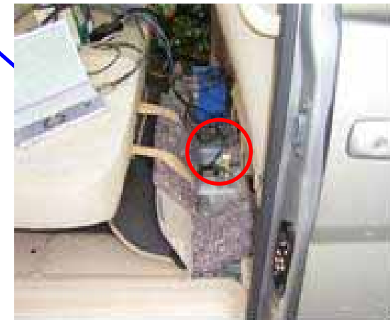
Accelerometer (installed at the middle of the body )
